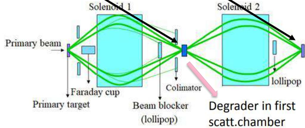
Second solenoid helps cleaning the secondary beam: degrader changes the  $B\rho$  of the particles with different  $Z$  ( $q$ )
