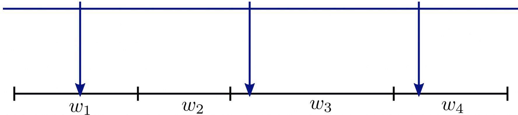
If there are  $K$  particles at the end of a time interval and the objective is to comb them to  $M$ , these  $K$  particles will be combed into  $M$  using a comb with  $M$  teeth.
