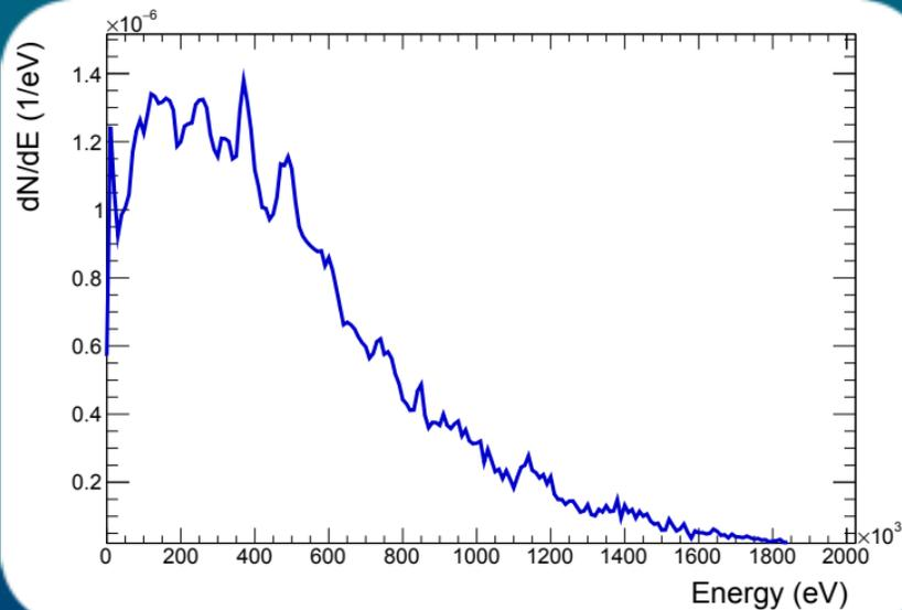
$^{235}\text{U}$  delayed fission neutron energy spectrum taken from ENDF-B/VIII.0
