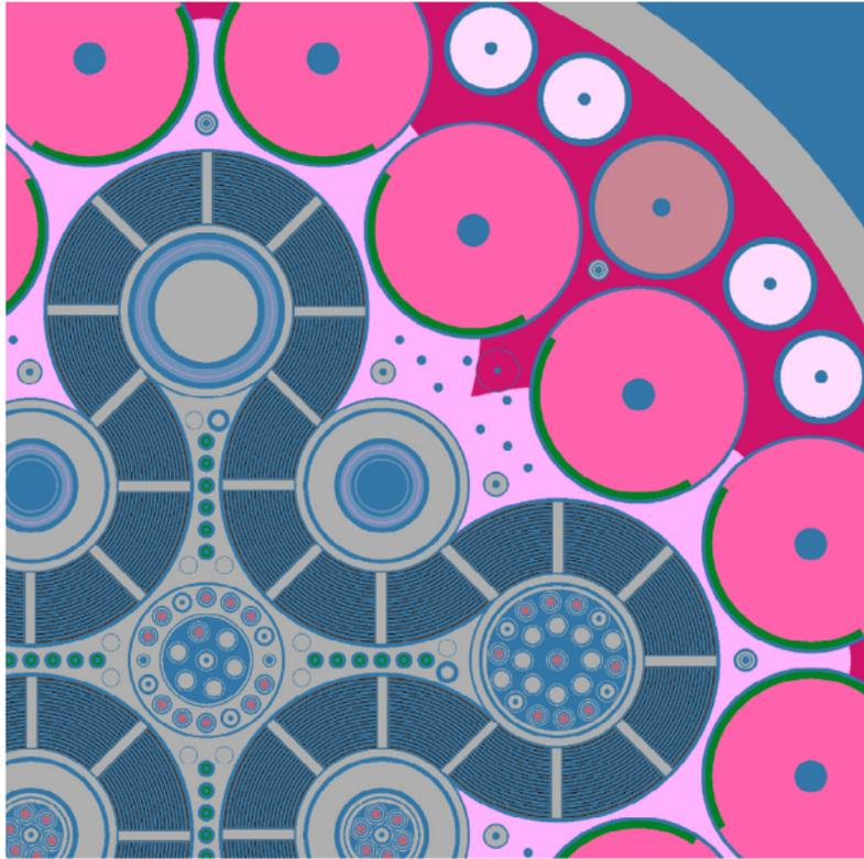
**Fig. 1.** Cross-sectional view of a section of an OpenMC model of the Advanced Test Reactor (ATR).
